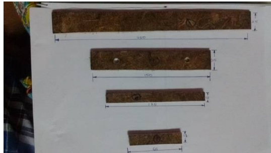
Fig 2 test specimens for tensile, compression, flexural, impact.
