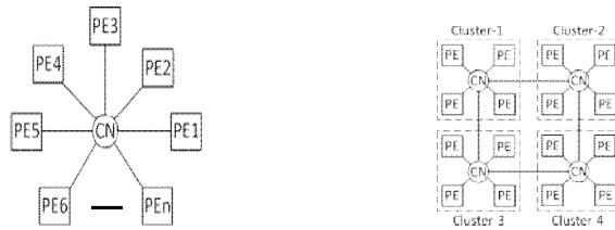
Fig 5. CDMA NoC scaling. (a) Directly scaling. (b) Cluster based scaling
