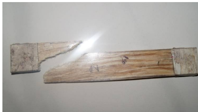
Fig. 6 Failed specimen after performing tensile strength
