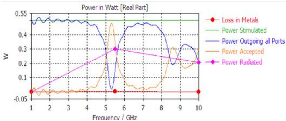
Fig 9. Power with Rogger RT 5880 substrate at 5.6GHz
