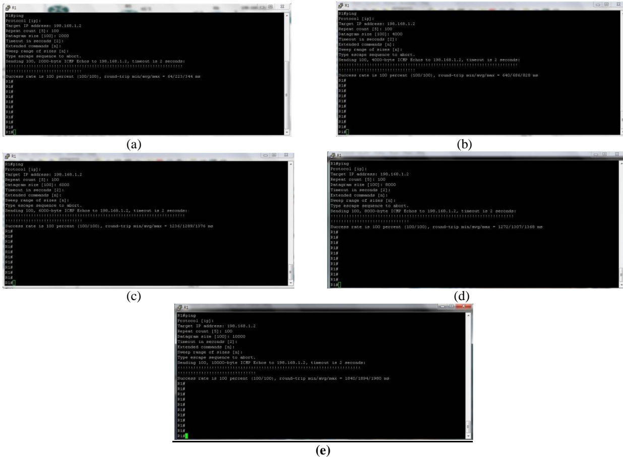
Fig 5: Response Time of the OSPF request (a) Time taken to send 2000 bytes (b) Time taken to send 4000 bytes (c) Time taken to send 6000 bytes (d) Time taken to send 8000 bytes (e) Time taken to send 10,000 bytes
