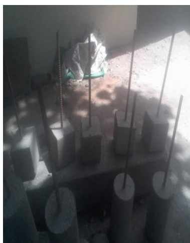
Fig. 2 Pull-out test specimens before testing
