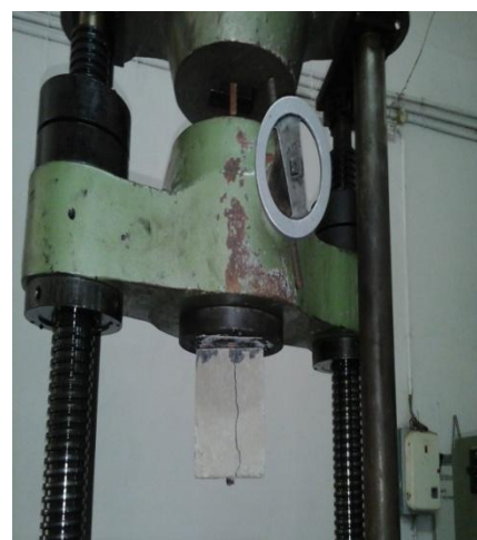
Fig. 3 Position of concrete cube for bond strength in UTM
