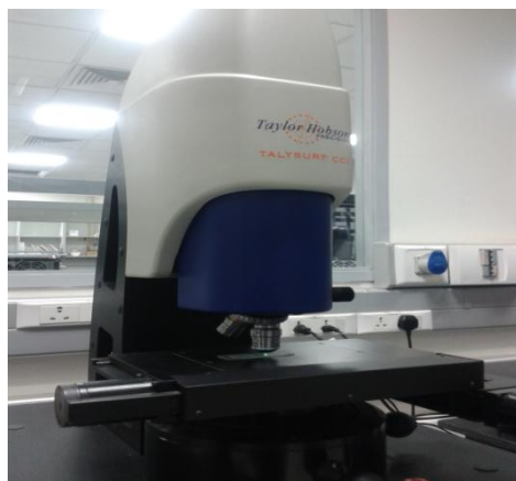
Fig 4.1- Optical Profilometer equipment for measuring Surface Roughness
