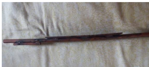
Fig.1: 1.25 cm diameter copper pipe welded with rectangular bar
