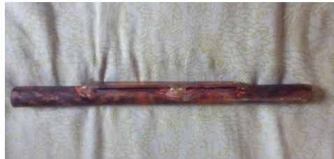
Fig.2: 2.54 cm diameter copper pipe welded with rectangular bar
