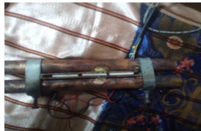
Fig.6: TEC1-12706 placed between 2.54cm diameter pipes
