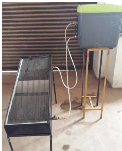
Fig 1: solar water heater without pebble stone
