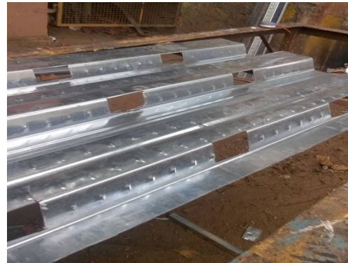
Fig 4: Corrugated steel sheet with holes
