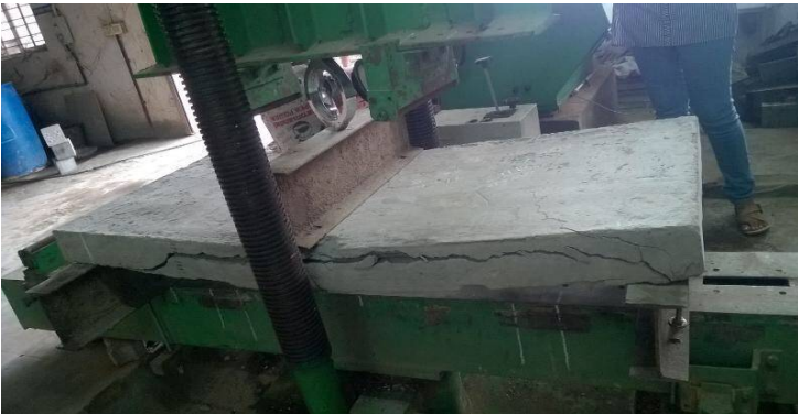
Fig 3: Bending test of the Panel
