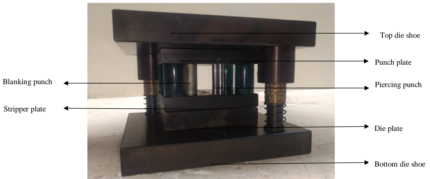
Fig. 4. Fabricated press tool
