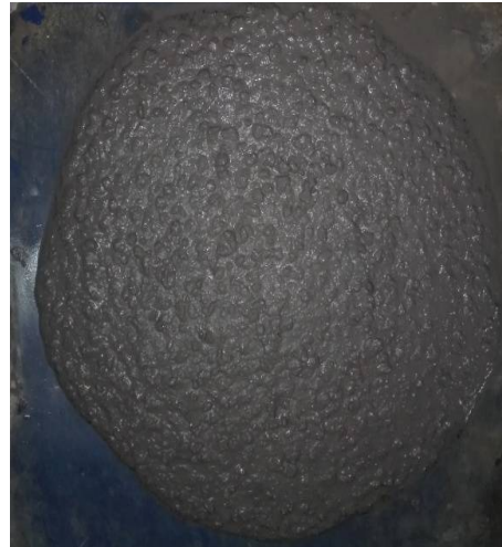
Fig.3 Slump flow test
