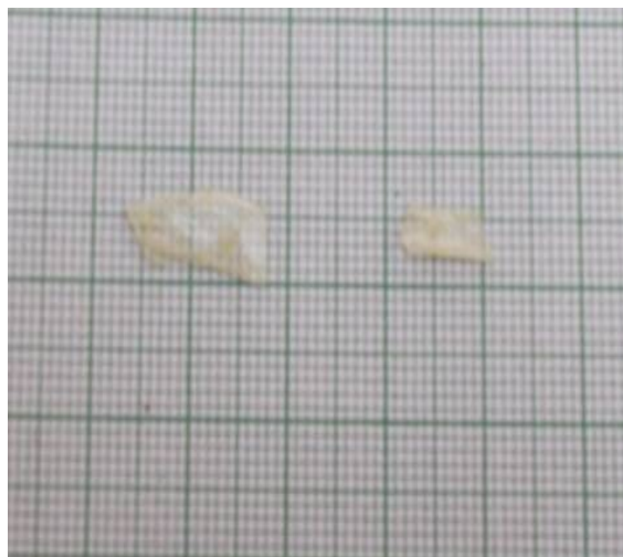
Fig (1) SA : FeSO 4 crystal grown by slow evaporation technique.
