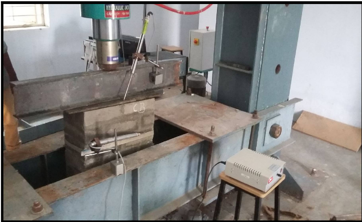
Test setup on wall panel
