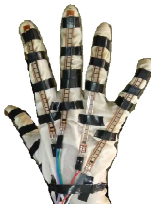
Fig. 5 Flex Sensors mounted on a Hand glove
