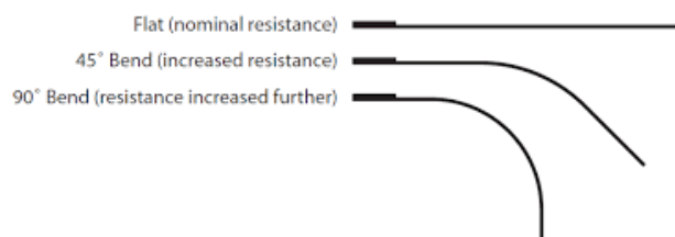
Fig. 2 Resistance Change Diagram [11]
