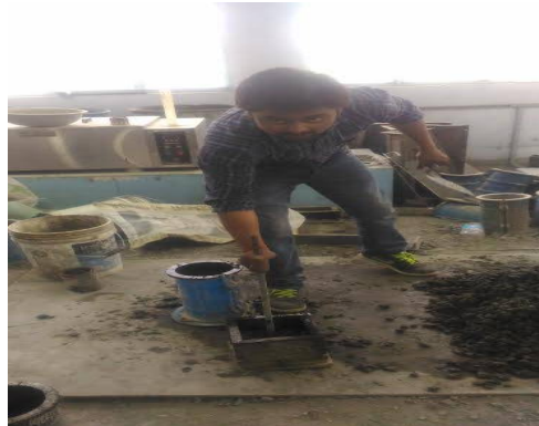
Casting a sample and compacted it.
