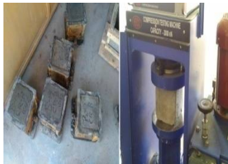
Figure 1- Testing of Cube
