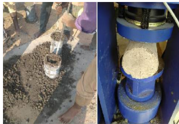
Figure 4 -Testing of Cylinder
