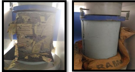
Fig.2 RC column showing crack patterns and CFFT Column showing buckling effect on axial load test under compressive testing machine.
