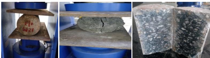
Figure 2: Split Tensile Test
