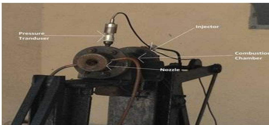
Fig.7:Hybrid Rocket Static Test Firing Set-up
