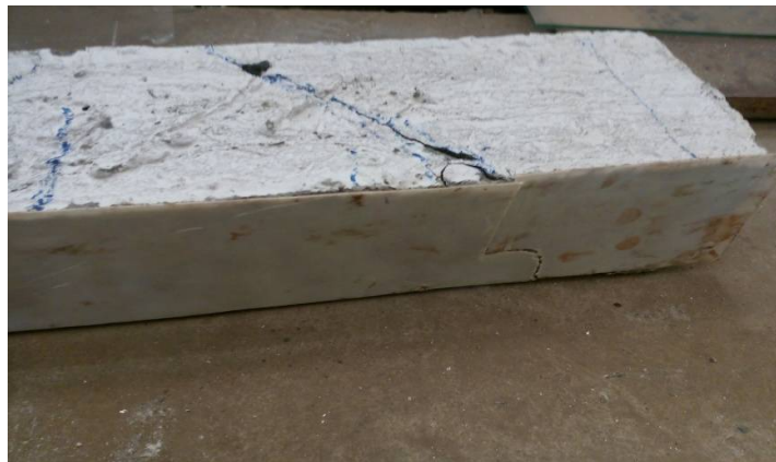
Fig. 6 GFMIX Beam with GFRP SHEET
