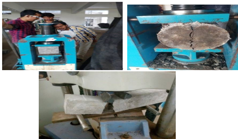
Fig 4: Experimental pictures (compression, tension, flexural tests)
