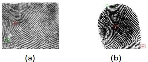
Fig 9 Singular Points Detection (i.e. Core & Delta) did for (a) NIST SD4 Fingerprint (b) FVC 2002 Fingerprint.
