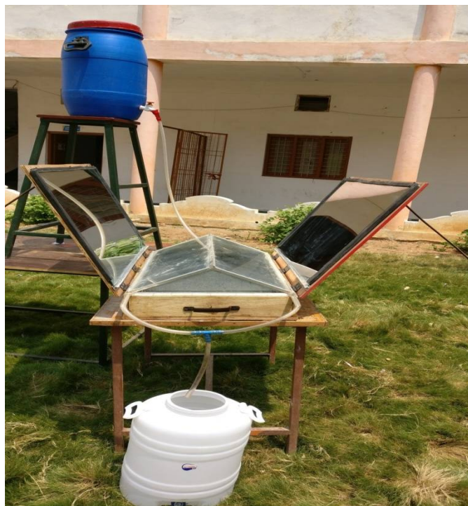
Fig V.I: Fabricated Double Slope type Solar Still with External Reflecting Mirrors
