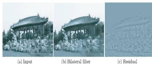
Figure 9: Filtered and residual image by Bilateral Filter
