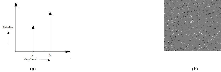
Figure 3: (a) probability density function of "salt and pepper" noise (b) "salt and pepper" noise when introduced into an image.
