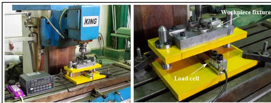
Figure 5: Axial load measuring rig
