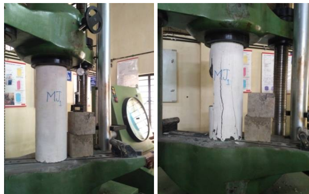
Fig.6. Testing of Micro Concrete Jacketed Column (a) Ready for testing (b) After failure at ultimate load
