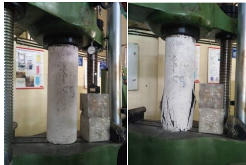
Fig.5. Testing of Conventional Concrete Jacketed Column (a)Ready for testing(b) After failure at ultimate load
