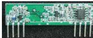
Fig 7. 315/434 MHz Ask Receiver
