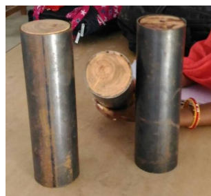
Fig 3. Timber filled with steel tube.
