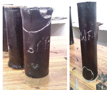
Fig 7: Failure mode of CFRP wrapped specimens
