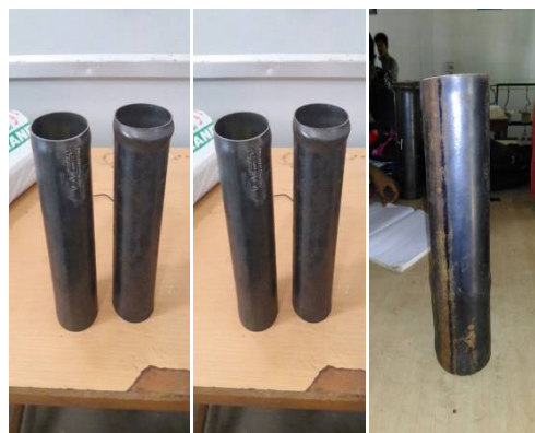
Fig 6: Failure mode of bare tubes
