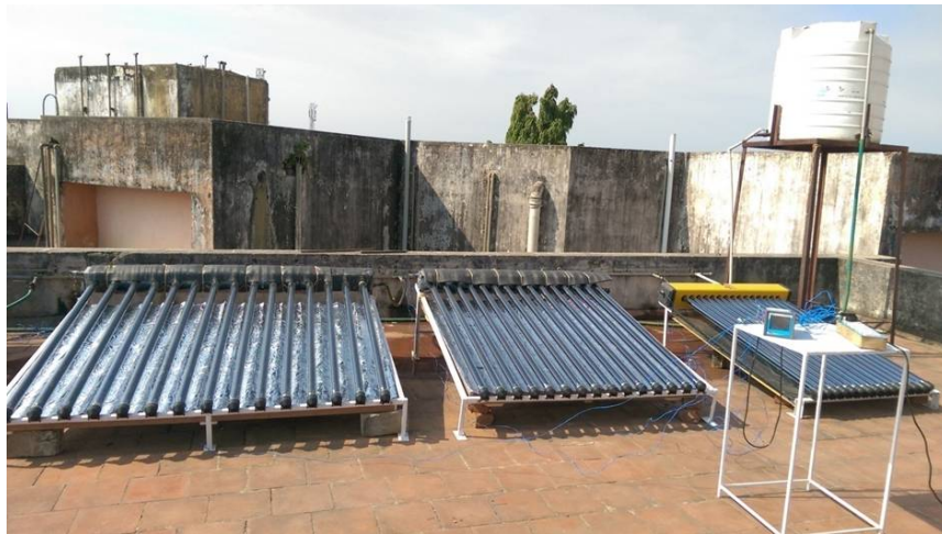
Fig.2 The evacuated U-tube solar collector under study.
