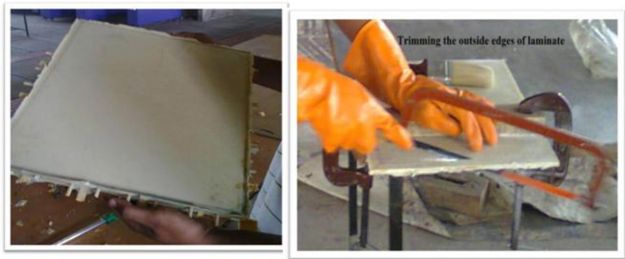
Fig 3.12: Trimming the edges of Cured Laminate
