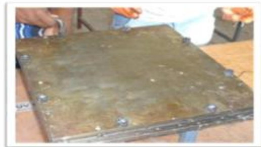
Fig 3.8 : Placing punch plate & clamping
