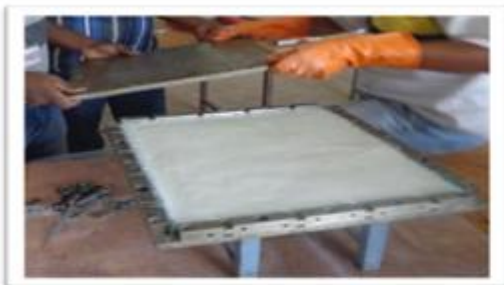
Fig 3.8 : Placing punch plate & clamping
