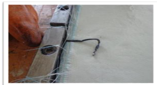
Fig 3.6: Placing the Thermocouple Bead
