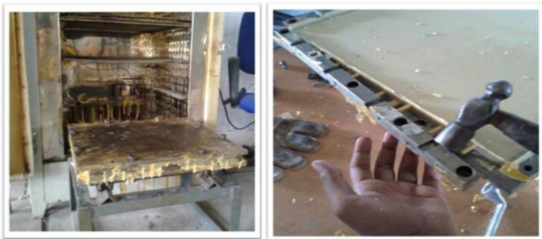
Fig 3.11: Removing the cured laminate
