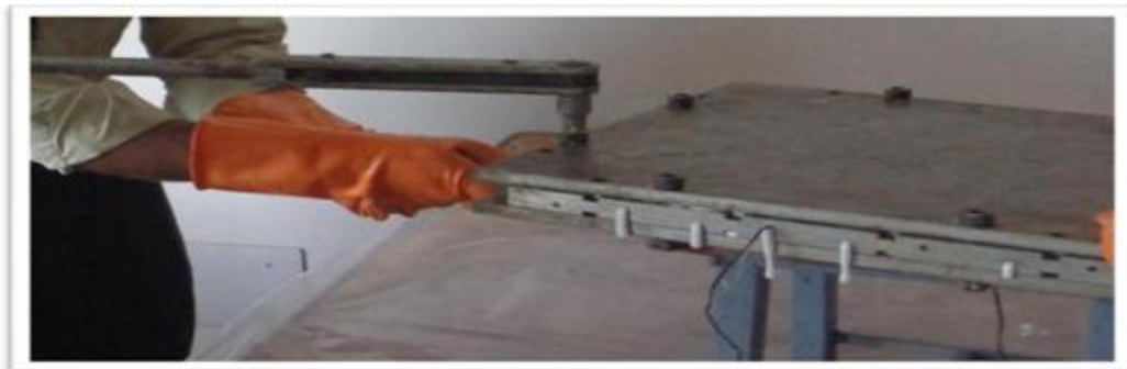
Fig 3.9: Applying tightening torque on the clamping bolts of the moulds.
