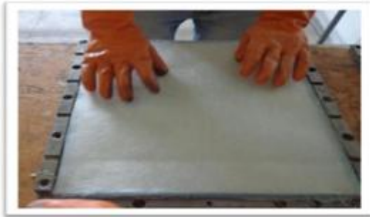
Fig 3.7: Placing the Last Layer (Surface mat)
