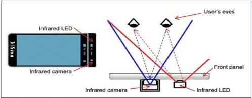
Fig 1: Iris Scanning by Biometric Machine
