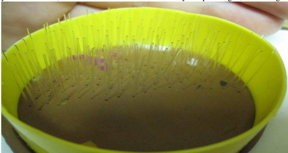
Fig 5. The figure shows placing of fibres. Place the fibres carefully in order to avoid displacement of fibres.
