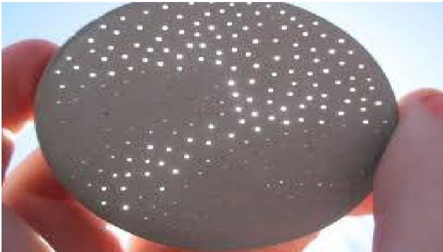
Figure 6. Thoroughly polish the surface of the model by using sand paper so that it can produce a light transmitting effect.
