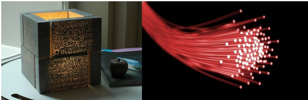
Fig. 1. Light passing through translucent concrete using optical fibre.
