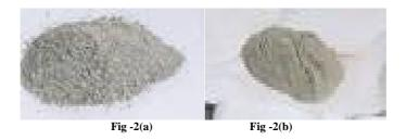
Fig - 2(a) shows IS Sieve 300 $\mu$  retained Quarry Dust passing through IS Sieve 600 $\mu$  and Fig - 2(b) shows IS Sieve 150 $\mu$  retained Quarry Dust passing through IS Sieve 300 $\mu$ .
