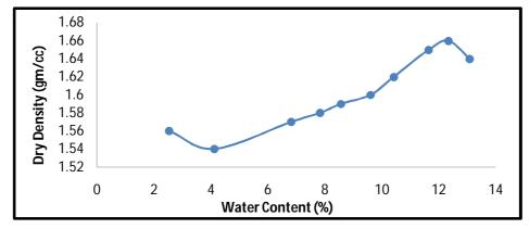
Figure 2: Variation of Dry Density with Moisture Content
