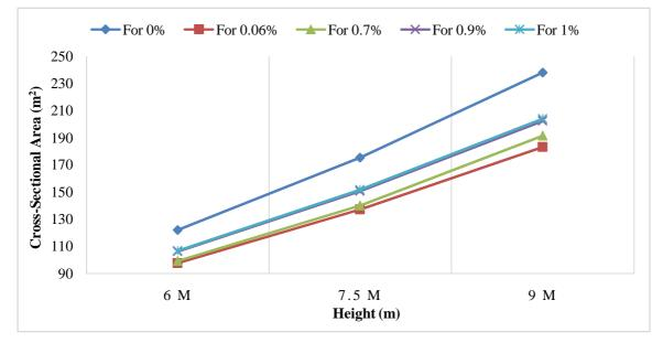
Figure 6: Variation in Cross-Sectional Area of Road Embankment with its Height for Mix Compositions of Different Percentages by Weight of Polybags Waste Material mixed with Dune Sand of 1.62 gm/cc Dry Density
