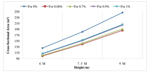
Figure 5: Variation in Cross-Sectional Area of Road Embankment with its Height for Mix Composition of Different Percentage by Weight of Polybags Waste Material mixed with Dune Sand of 1.57 gm/cc Dry Density
