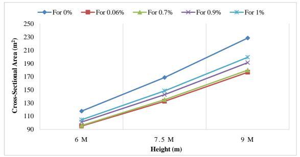
Figure 7: Variation in Cross-Sectional Area of Road Embankment with its Height for Mix Compositions of Different Percentages by Weight of Polybags Waste Material mixed with Dune Sand of 1.66 gm/cc Dry Density
