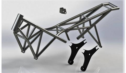
Fig.1: Exploded View of Trellis Frame and Components
