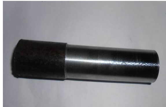
Fig 3.2: Work piece after turning
