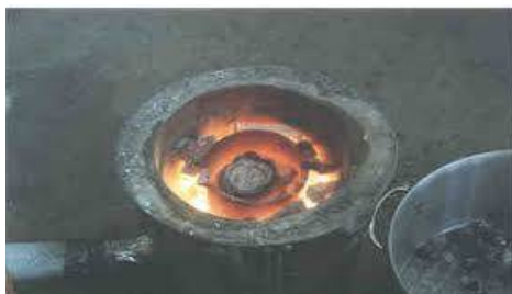
Fig 3.3.2: crucible inside the furnace
