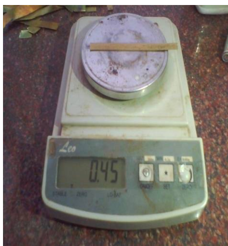
Figure 8: Digital weighing machine and soaked fibres in water
