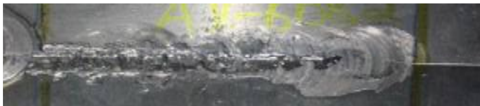
Fig. 4.3: Trial 1 of Welded Soft Steel/Mild Steel & AA6082 – T6
