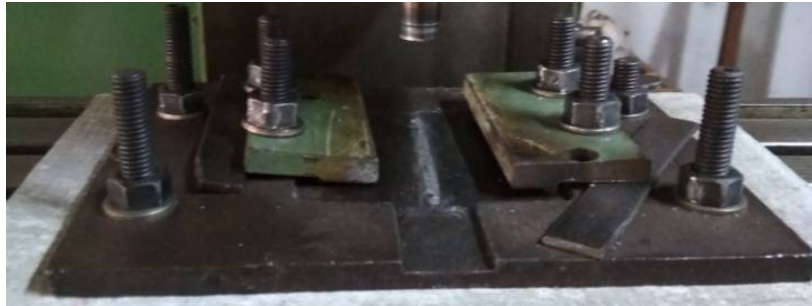
Fig. 4.1: Fixture to hold the Workpieces
