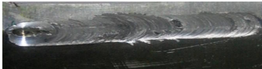
Fig. 4.10: Trial 8 of Welded Soft Steel/Mild Steel & AA6082 – T6
