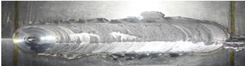
Fig. 4.4: Trial 2 of Welded Soft Steel/Mild Steel & AA6082 – T6
