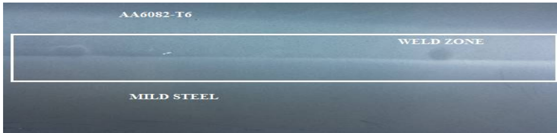
Fig. 5.1.3: Radiography Film Image of Trial 8 Welded Specimen
