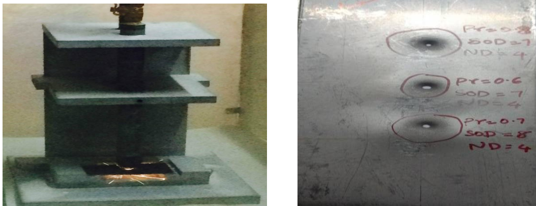
Fig 1. Shows the machining of Hastelloy using AJM and the Hastelloy machined based on L9 orthogonal array
