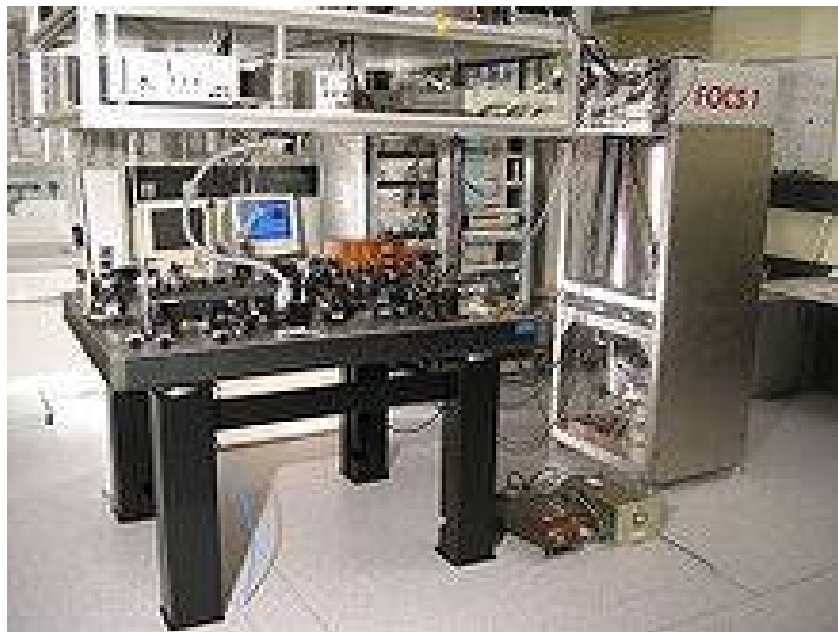
Fig.23 The FOCS-1, a continuous cold caesium fountain atomic
