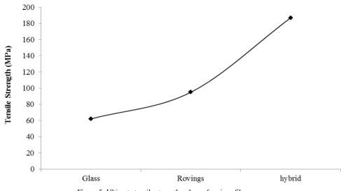
Figure 5: Ultimate tensile strength values of various fibers
