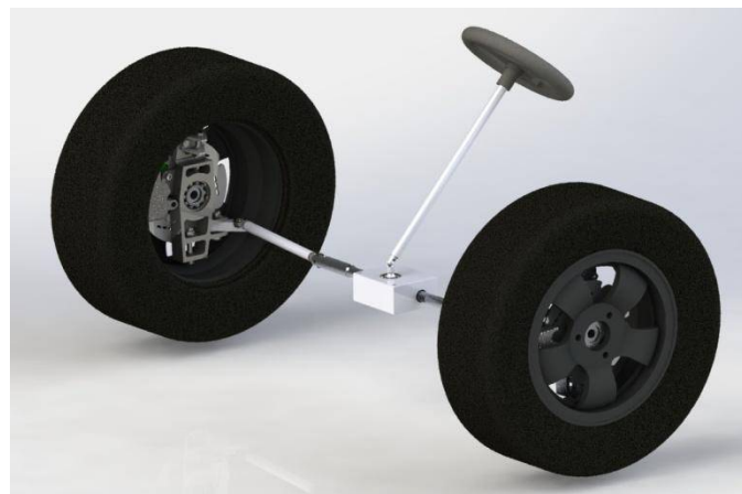
Fig 4. Rack and pinion assembly as seen in Solid Works
