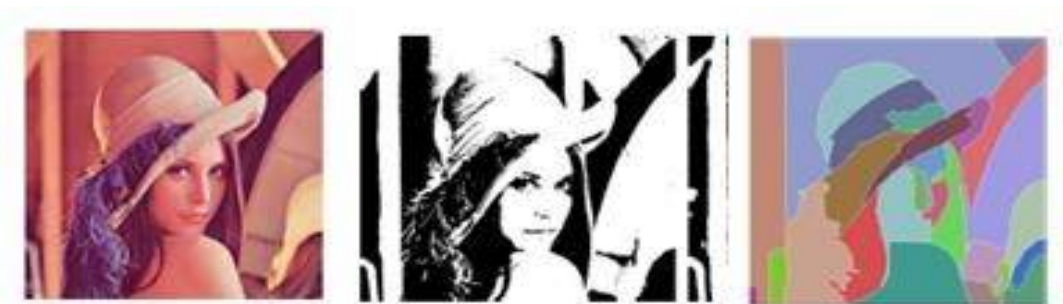
Fig.8 i) Lena-color scale input image ii) Otsu based threshold image iii) Watershed Segmented image
