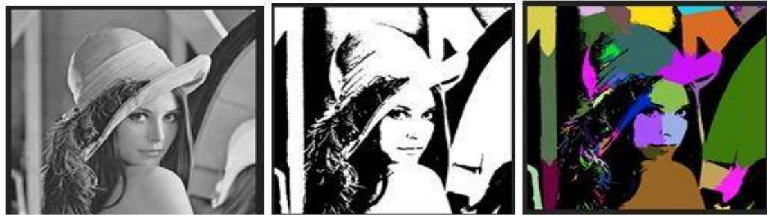
Fig.4 i) Lena-grey scale input image ii) Otsu based threshold image iii) Watershed Segmented image
