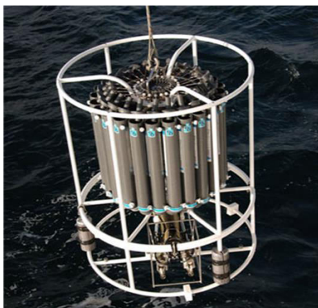
Fig 6.3: A CTD is brought into the dilute to gauge the saltiness, temperature, profundity and convergence of particles in the water section.
