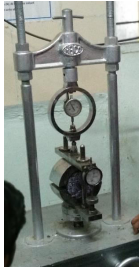
Fig7: Mould being tested for Stability and flow
