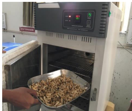
Fig1: Cigarette butts placing in the oven at 105°C for 24 hours
