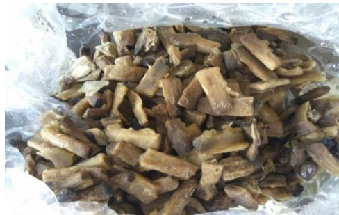
Fig 4: Cigarette butts encapsulated with wax cooled
