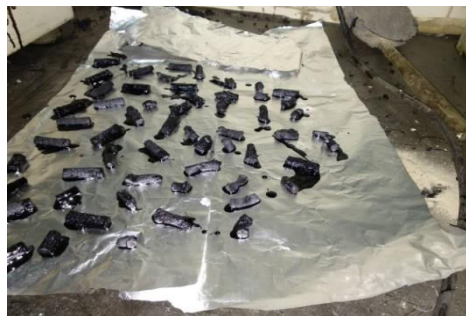
Fig 2: Cigarette butts encapsulated with bitumen left to cool
