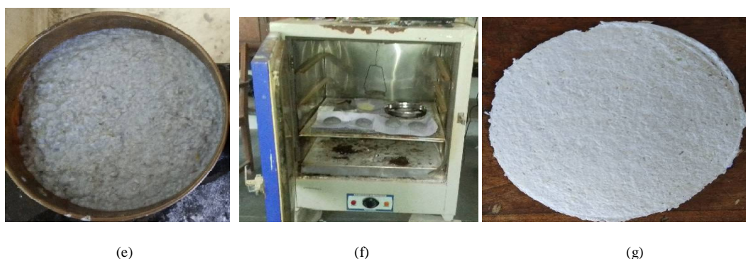
Fig. 5. Images of Chemical Deinking Methodology. (a)- Pulping Stage (b)- Hyperwashing (c)- Flootation (d)- Bleaching (e)- Hand Sheet Preparation (f)- Oven Drying (g)- CD-101
