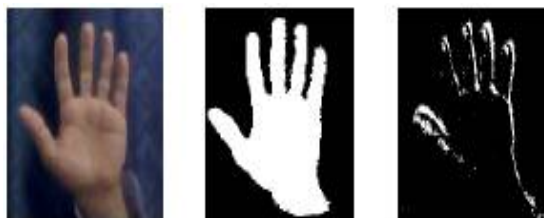
Fig 2. (a) Original hand detected image, (b) Skin color region, (c) Combination of skin and motion pixels [10].
