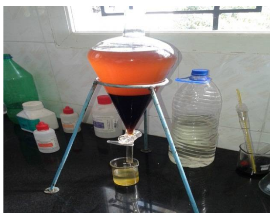
Fig 2 Separation of glycerin and biodiesel
